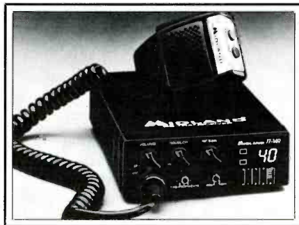
The Midland Model 77-149 offers channel selection buttons on the mike.
