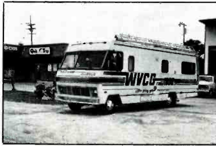
The mobile studio of WVCG (1080 kHz), Coral Gables, FL. The vehicle sports a 50-ft. telescoping tower made by Aluma Tower Company, Inc., Vero Beach, FL. (Courtesy Aluma Tower Company.)
