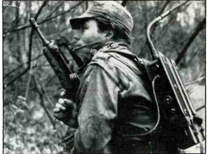
The French military TRC559 military manpack transceiver operates with NBFM with channels spaced 25 kHz apart between 30 to 80 MHz.
